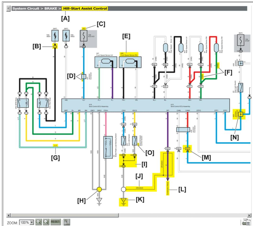
**[M]:**Indicates the code for the (male and female) connectors which are used to join two wire harnesses. The connector code consists of two alphabetical and one numerical characters.
