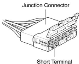
Junction connector in this manual include a short terminal which is connected to a number of wire harnesses. Always perform inspection with the short terminal installed.
